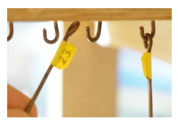
Hang the wire with its eye going over the hook on the bottom of the windbox.
